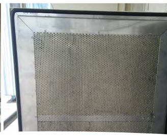
16-gage 304SS internal liner protects high-temperature acoustic insulation.
