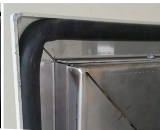
High-temperature replaceable gasket.
